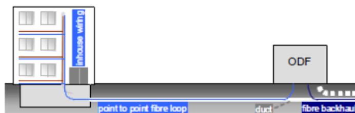
Point-to-point FttH design (BoR (10) 08, Ch. B.2.1.1)
